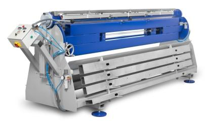
The material to be bent is cut to size and aligned with the machine's stops. The fusion process is started with a 2-hands button and the fusion unit moves over the panel material. The fusion unit moves away from the material at the end of the fusion time. The process head, consisting of the fusion unit and ejection section, is swivelled manually around 180° and the heated and plasticized material is pressed into the receiving shaft to shape the profile after the 2-hands
